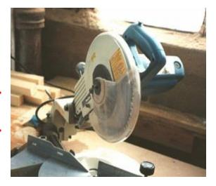
This miter saw has a blade that needs to be cleaned of excess sap. This caused kickback of the wood. 1910.213(s)(1)
