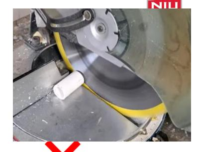
This pvc pipe is not clamped down and could kick back. Section 5(a)(1)
