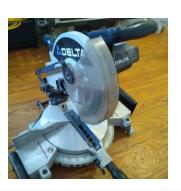
This hand is within 6 inches. Lower blade guard is missing.
