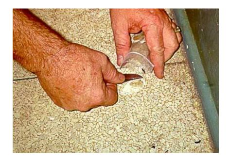
Sample of a tile scraped to be tested.
